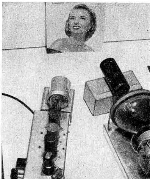
Arrangement for reflection scanning of opaque material. A 3 in. diameter plano-convex condenser lens is used in front of the photocell on the left. The 5FP7 scanning tube with its 5 in. focal length lens is on the right.
